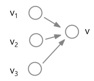
$$w(v) = H(v || w(v_1) || w(v_2) || w(v_3))$$
